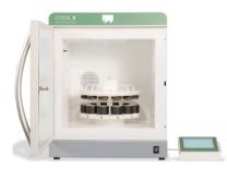
Microwave-assisted solvent extraction offers superior lab efficiency in the determination of organic pollutants with microwave green extraction technique. Typical applications include chlorinated pesticides, semivolatile organics, PAHs, PCBs, chlorinated herbicides, phenols, organophosphorus pesticides, dioxins and furans.
