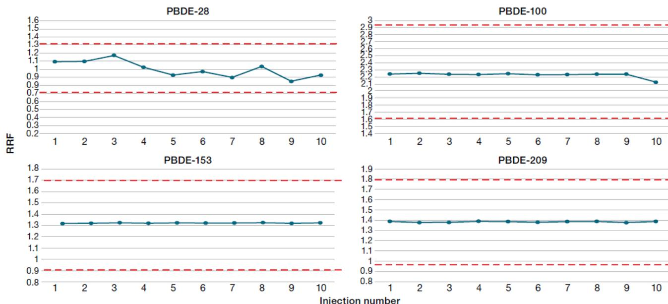
**Figure 6.** Examples of the consistency of the RRF for some selected PBDEs. The RRF was within  $\pm 30\%$  of that calculated from the average of the calibration. The amber dotted lines represents the acceptance limits.
