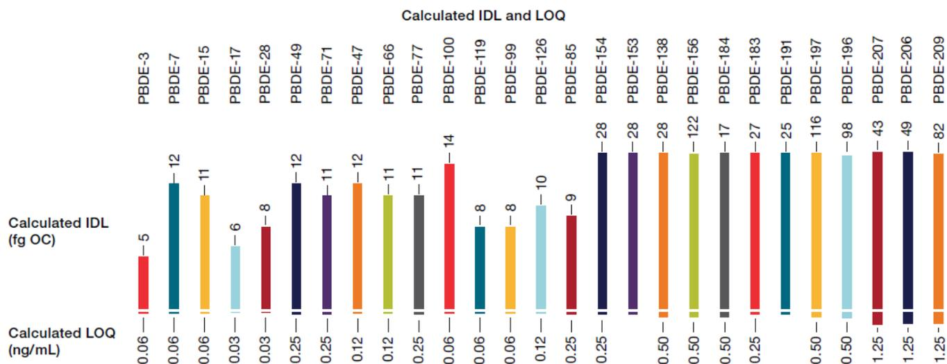
**Figure 5.** Calculated IDLs and LOQs for all investigated PBDEs. Calculated IDLs ranged from 5 fg to 122 fg on column (OC), corresponding to 0.25 pg/L to 6.10 pg/L for water samples and 0.025 to 0.61 ng/kg for soil and fish oil samples. Calculated LOQs ranged from 0.03 to 1.25 ng/mL, corresponding to 1.5 pg/L to 62.5 pg/L in water samples and 0.15 to 6.25 ng/kg in soil and fish oil samples.
