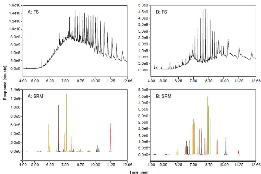
**Figure 3.** TIC (FS:  $m/z$  40–1,000) and SRM acquisitions for environmental (A-left traces) and fish oil (B-right traces) sample extracts containing PBDEs showing the complexity of the matrices (FS acquisition) and the selectivity of the SRM acquisition.
