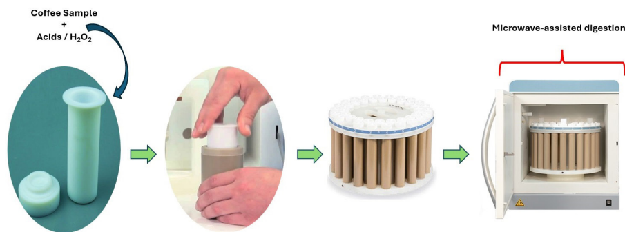
Figure 3. Microwave digestion procedure in closed pressurized vessel.
