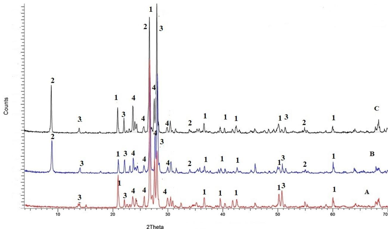
**Figure 6.** XRD spectra of the rocky supports from La Castreña (A), Boca del Álamo (B) and Cerro Pintada (C). The crystalline phases are: 1. Quartz, 2. Phlogopite, 3. Albite, 4. Anorthoclase.
