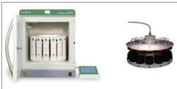
Figure 1. Milestone's ETHOS X with SR-15 extraction rotor (left) and RAR-15 evaporation rotor (right).
