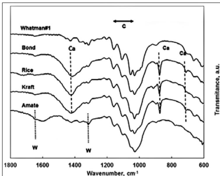
**Figure 3.** Infrared spectra of the papers exposed at 9 W. C: Cellulose, Ca: Calcite, W: Whewellite.
