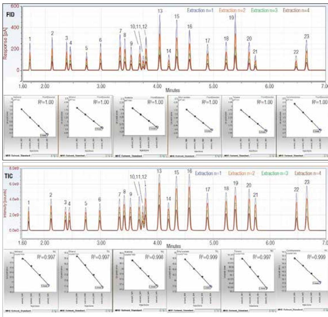
**Figure 1.** FID and TIC (full-scan, EI at 70 eV) traces for reference standard and corresponding MHE calibration curves for selected compounds (left to right: methanol, ethanol, acetone, ethyl acetate, toluene, and cyclohexanone) as examples. Calibration curves were obtained by plotting the natural logarithm of peak area responses (total vaporization MHE) versus the corresponding MHE extraction step.
