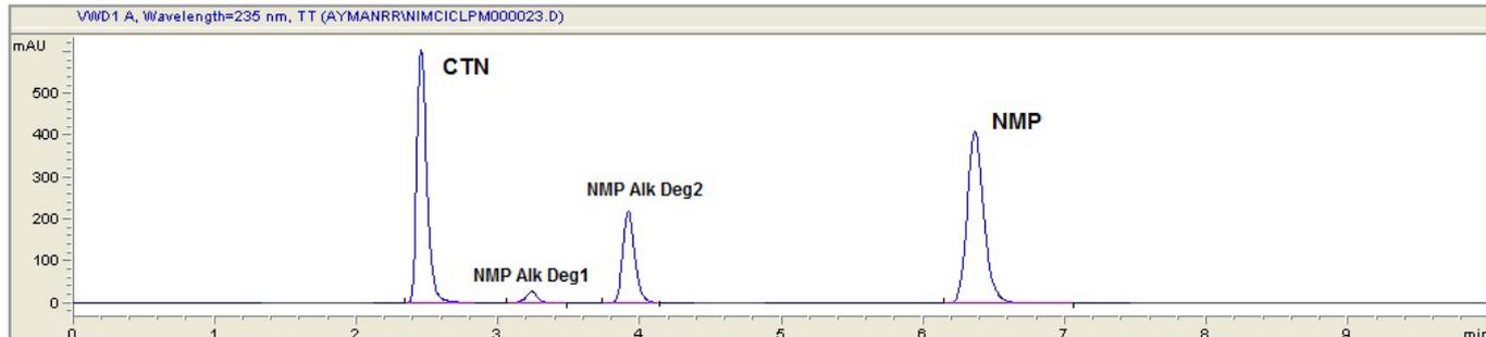
**Figure 3.** A typical HPLC chromatogram of synthetic ternary mixture of 150  $\mu\text{g mL}^{-1}$  citicoline sodium, 11  $\mu\text{g mL}^{-1}$  nimodipine alkaline degradates and 45  $\mu\text{g mL}^{-1}$  nimodipine
