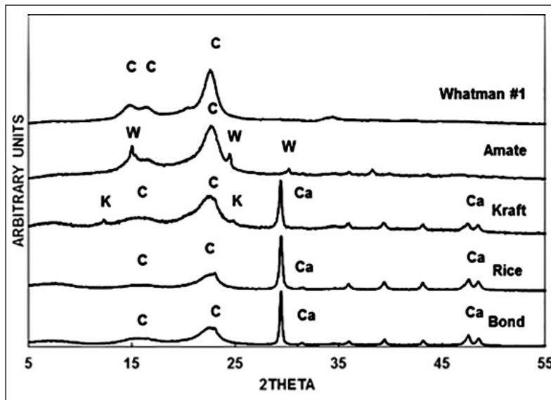
**Figure 2.** X-ray diffraction patterns of the papers. C: Cellulose, Ca: Calcite ( $\text{CaCO}_3$ ), W: Whewellite ( $\text{CaC}_2\text{O}_4 \cdot \text{H}_2\text{O}$ ), K: Kaolinite ( $\text{Al}_2\text{Si}_2\text{O}_5(\text{OH})_4$ ).
