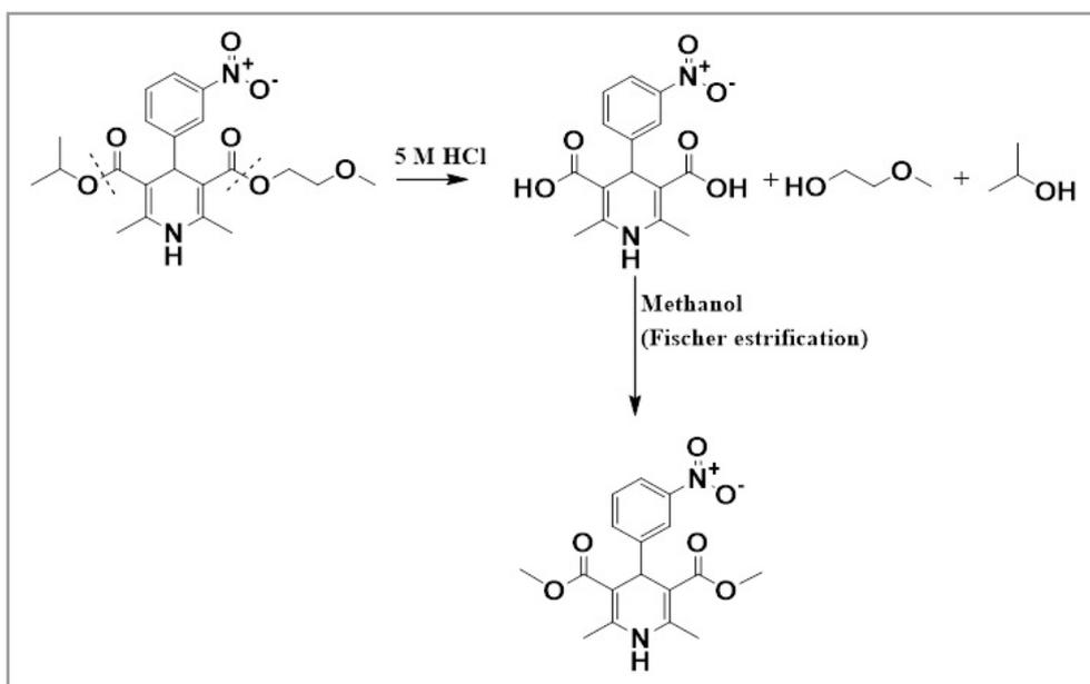
**Figure 4.** The suggested scheme for nimodipine acid degradation.
