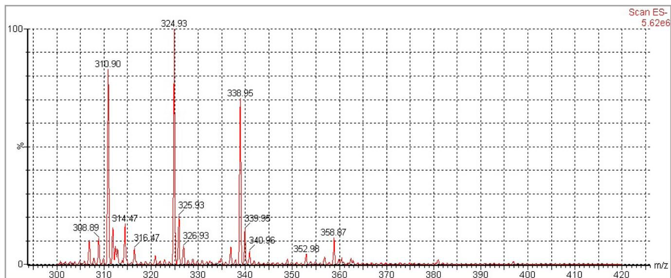
LC-MS/MS spectrometry of nimodipine alkaline forced degradation products
