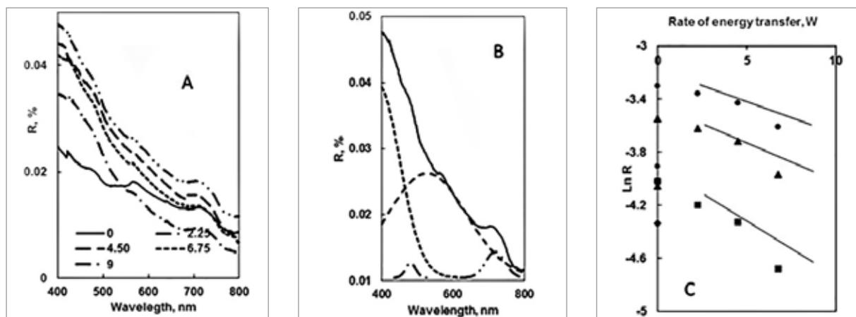
**Figure 6.** A: Visible diffuse reflectance spectra of kraft paper, exposed from 0 to 9 W. B: Deconvolution of the visible diffuse reflectance spectrum of kraft paper (exposed at 2.25 W). C: Behavior of  $\text{Ln R}$  as a function rate of energy transfer at 481 nm (circles):  $\text{Ln R} = -0.004 \text{ RET} - 3.1$  ( $R^2=0.92$ ), 527nm (triangles):  $\text{Ln R} = -0.005 \text{ RET} - 3.4$  ( $R^2=0.91$ ), and 718 nm (squares):  $\text{Ln R} = -0.008 \text{ RET} - 3.8$  ( $R^2=0.95$ ).
