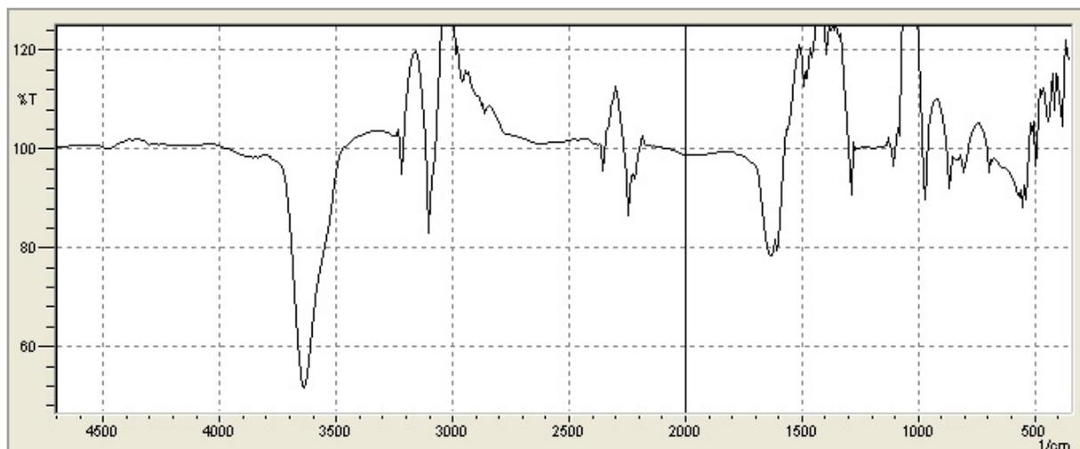
FT-IR spectrum of nimodipine alkaline forced degradation products
