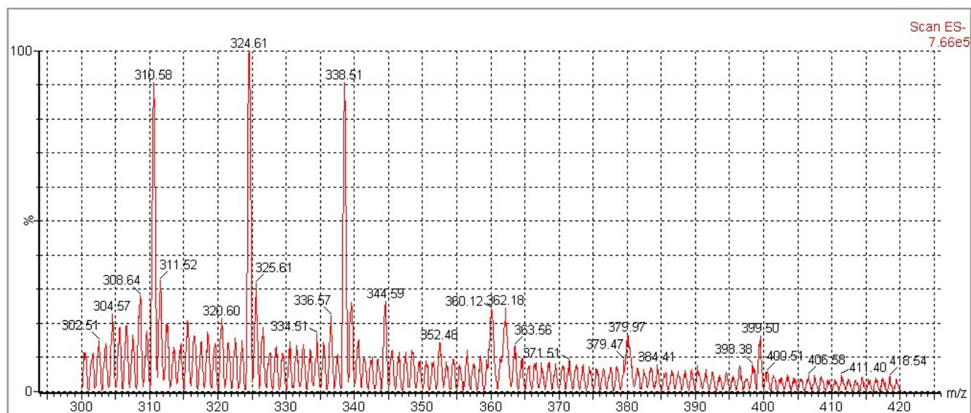
LC-MS/MS spectrometry of nimodipine acid forced degradation product
