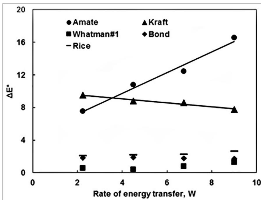
**Figure 7.** Colorimetric difference ( $\Delta E^*$ ) of the papers as a function the rate of energy transfer. For kraft:  $\Delta E^* = -0.25 W + 10.1$  ( $R^2 = 0.95$ ) and for amate:  $\Delta E^* = 1.3 + 4.7$  ( $R^2 = 0.98$ ).
