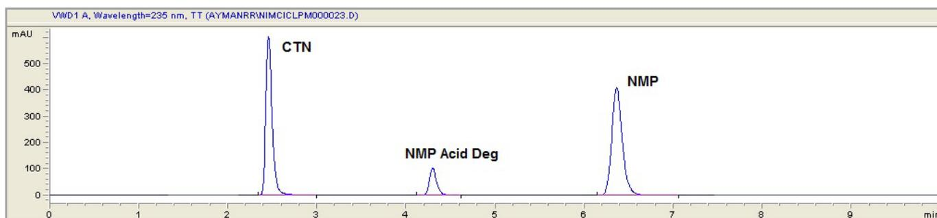
**Figure 2.** A typical HPLC chromatogram of synthetic ternary mixture of 150  $\mu\text{g mL}^{-1}$  citicoline sodium, 9  $\mu\text{g mL}^{-1}$  nimodipine acid degradate and 45  $\mu\text{g mL}^{-1}$  nimodipine.
