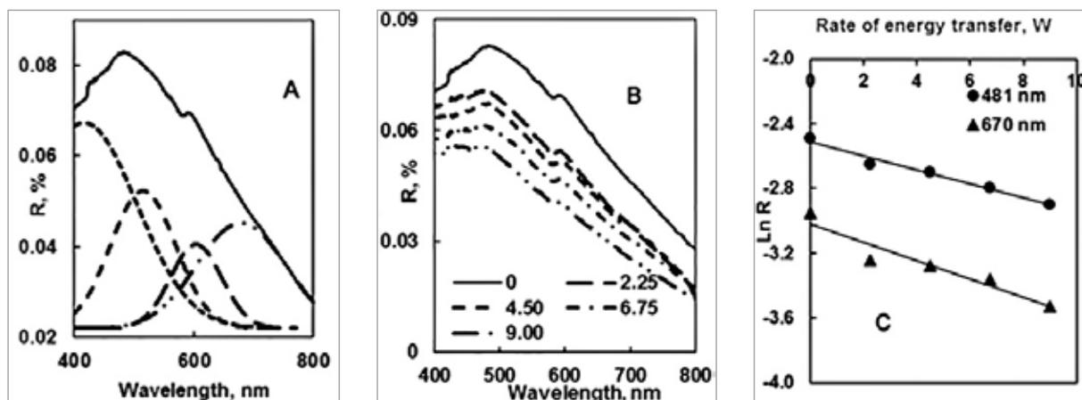
**Figure 5.** A: Deconvolution of Visible diffuse reflectance spectrum of amate paper. B: Visible diffuse reflectance spectra of amate paper, exposed from 0 to 9 W. C: Behavior of the  $\text{Ln R}$  as a function the rate of energy transfer at 481 nm (circles),  $\text{Ln R} = -0.005 \text{ RET} - 2.5$  ( $R^2 = 0.99$ ) and 670 nm (triangles),  $\text{Ln R} = -0.006 \text{ RET} - 3$  ( $R^2 = 0.96$ ).
