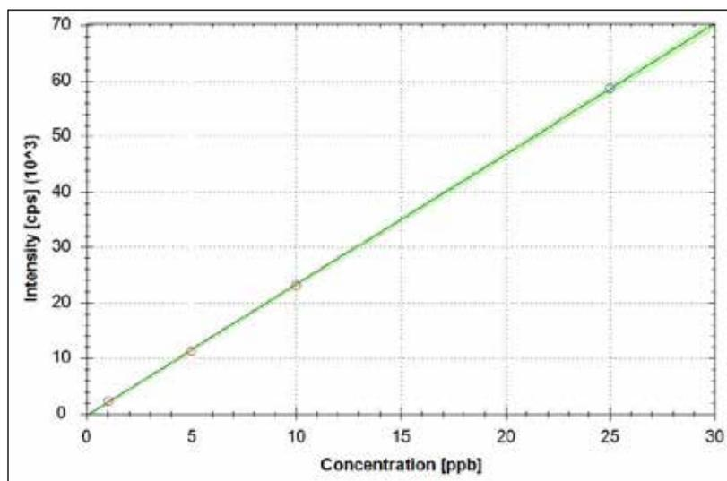
**Figure 1.** Calibration curve for bromate standards measured at <sup>79</sup>Br in He-KED mode.
