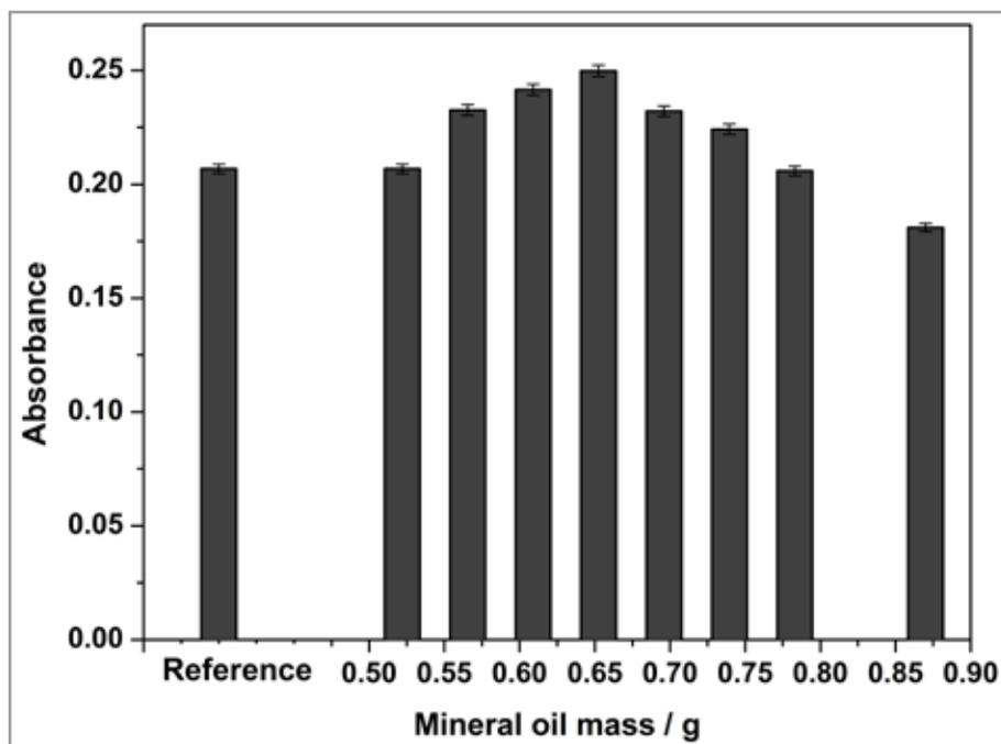
**Figure 2.** Evaluation of mineral oil mass added to the microemulsion for calibration. All systems contain  $2 \text{ mg L}^{-1}$  Cu,  $300 \mu\text{L}$  of aqueous phase ( $1.4 \text{ mol L}^{-1} \text{ HNO}_3$ ) and *n*-propanol (up to 10 mL). Reference: instead of mineral oil, this system contains 3.3 g of B7-diesel oil.
