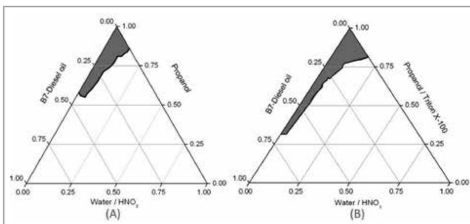
**Figure 1.** Ternary phase diagrams of B7-diesel oil, water/HNO<sub>3</sub> and *n*-propanol at 25 °C: (A) without Triton X-100 and (B) with 13% (w/w) Triton X-100. The component content in the system is in mass fraction. Microemulsion region is highlighted in gray.
