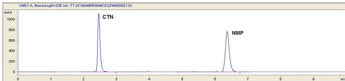
A typical HPLC chromatogram of Nimodilat plus® sample solution ( $305 \mu\text{g mL}^{-1}$  CTN and  $91.5 \mu\text{g mL}^{-1}$  NMP)
