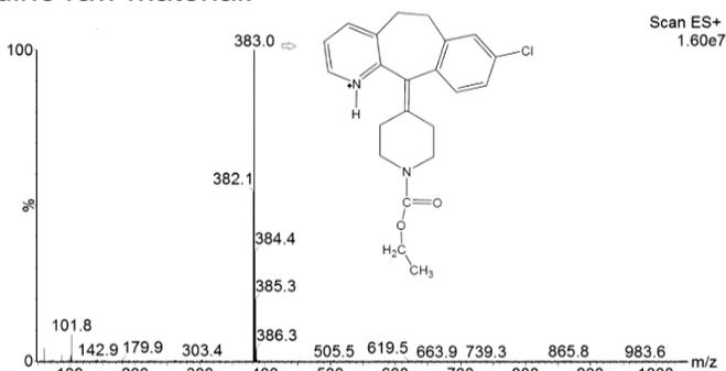
**Figure 6.** Mass Spectrum scanning of loratadine raw material with white appearance.
